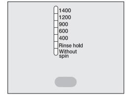
Press the "Spin" button repeatedly until the indicator light for the spin speed you want comes on.
